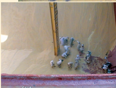
◀ Fig. 3: Although it is dangerous to work this close to the rotating part of the unloader chain, clean space must be available for the payloader.
