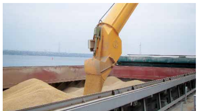
Fig. 3 (above) and Fig. 4 (below) shows 800tph loading spouts with 40m long reach.
