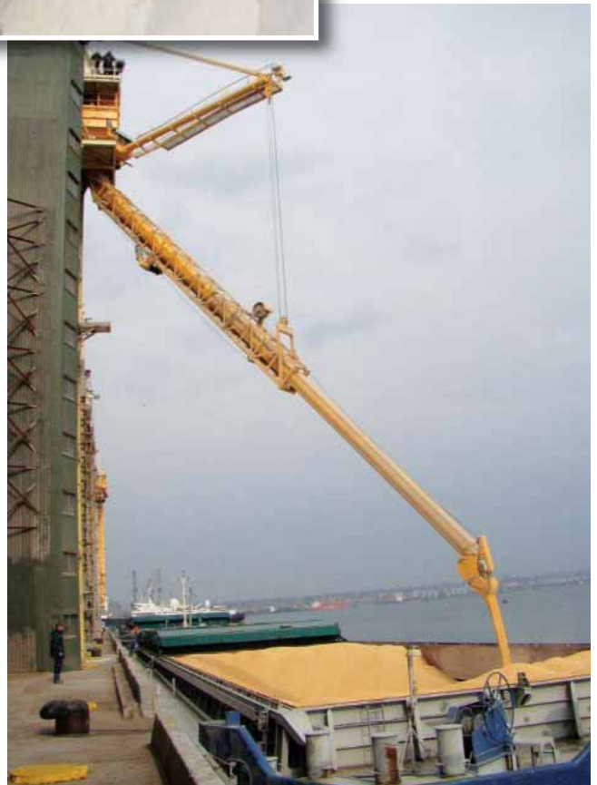
Fig. 3 (above) and Fig. 4 (below) shows 800tph loading spouts with 40m long reach.
