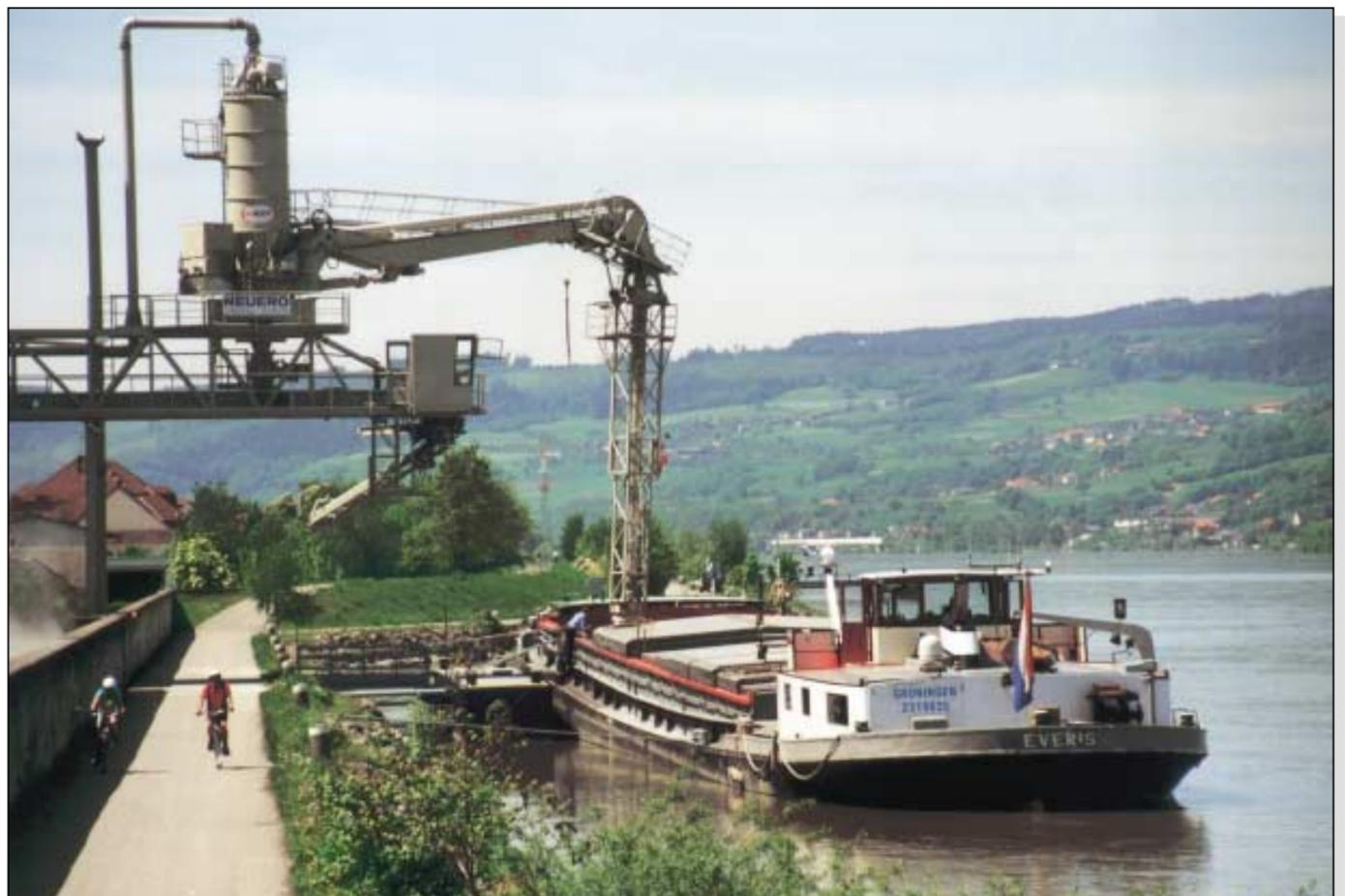
compensated for by using a hopper. The grab and the hopper must be large because of the low specific weight of the material handled. This hopper must also be equipped with an efficient dedusting system.
