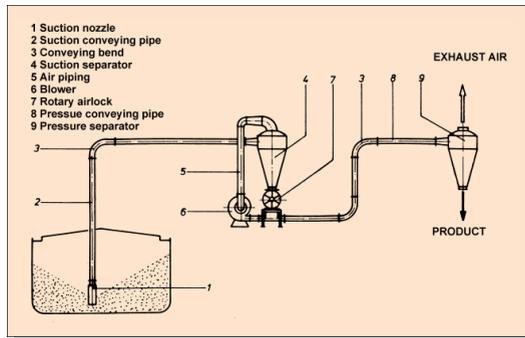
Pressure only systems are recommended when the product is introduced at one point, and optionally, using diverter valves (4) transported to different delivery points. Due to the higher pressure differential and specific weight of the air, they have a greater capacity than the suction type.
