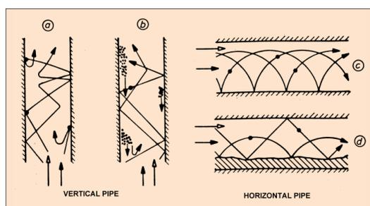
The necessary air speed  $w$  is called the suspension speed  $w_s$ . The minimal condition for conveying is that the air speed in a vertical pipe is higher than the suspension speed, and the difference is the real speed of each particle relative to the pipe. Thus:
