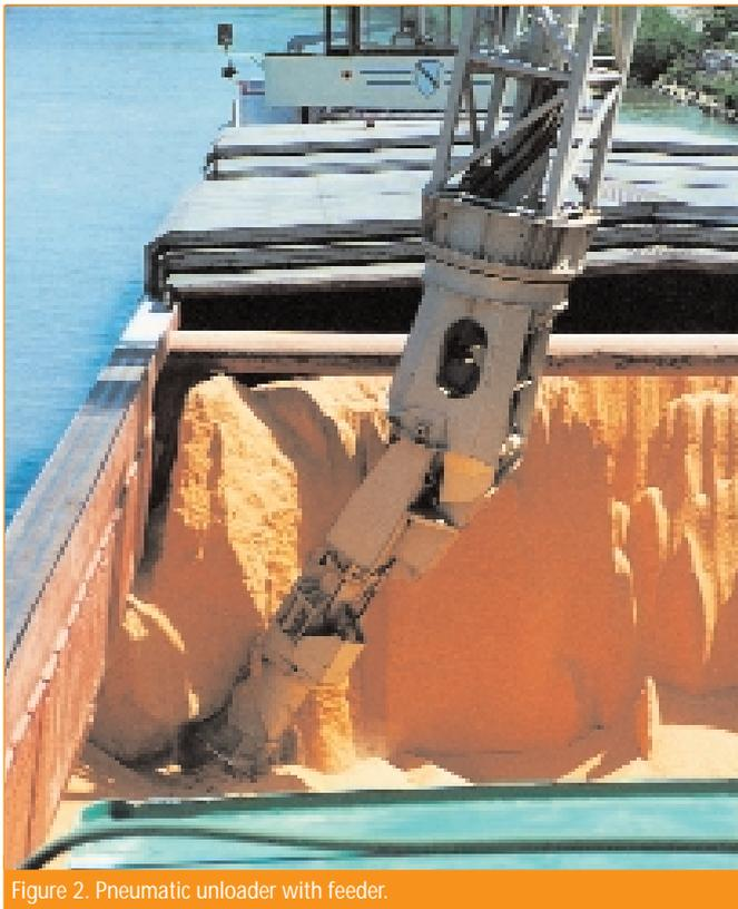
Figure 2. Pneumatic unloader with feeder.
