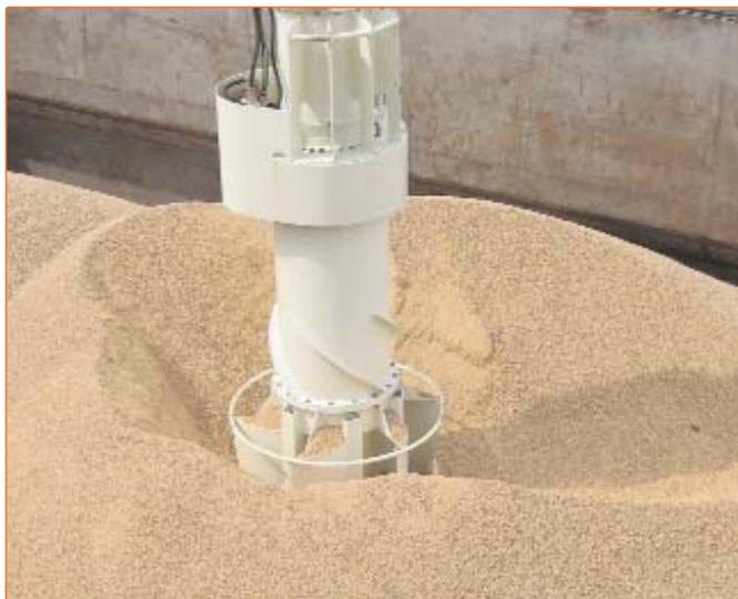
Figure 2. Rotating feeder.
