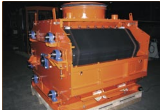
Figure 7. Assembled form showing the External bearings of the belt idlers.
