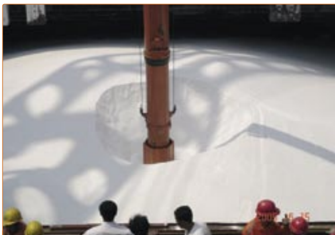
Figure 2. Each M300AL has a capacity of 300t/h.
