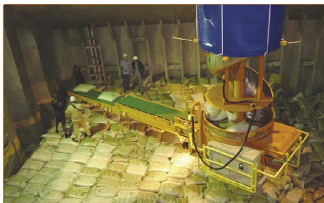
The head rotates by approx. 270° and can reach 360° with the telescopic rotating movement of the spiral chute. It has telescopic belts that are adjusted in order to place the bag close to empty space.
