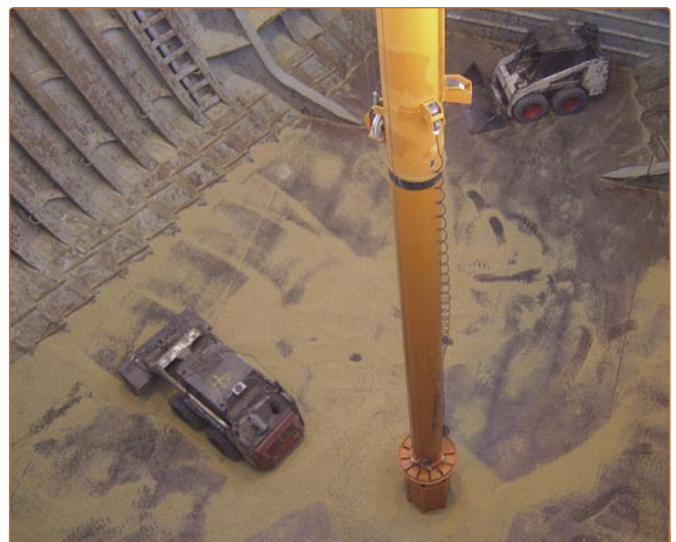
Figure 4. Pneumatic nozzle removes material from the hatch bottom.
