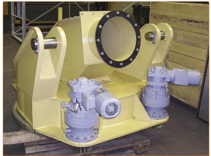
Figure 3. Curved chute designed to slow down the material.
