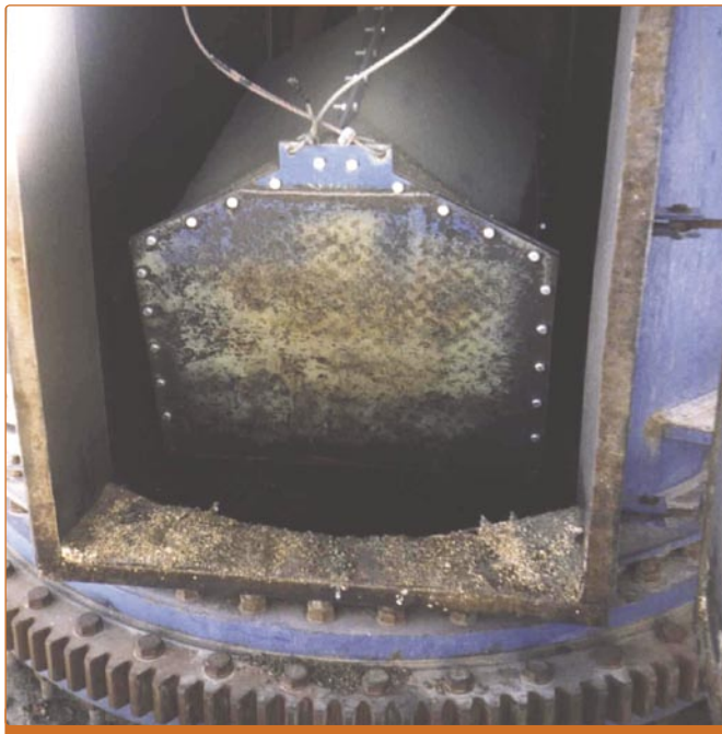
Figure 2. Unloading installations in the past did not pay proper attention to material breakage.
