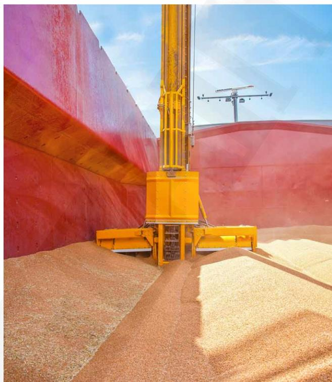
The Bargolink's marine leg is equipped with a fixed mounted feeding screw that digs into the grain in the ship's hold and lifts it up onto a horizontal chain conveyor that carries the cargo to the port's storage units. Photo courtesy of Bühler.
